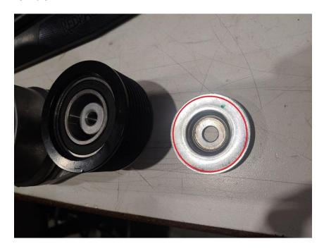
Using a shop press, press out the existing bearing in the steel pulley supplied with your Gates tensioner. **PRESS ONLY BY THE OUTER RACE!!!! Do not, I REPEAT, DO NOT** press the bearing out by its inner race, or you will destroy the bearing.
